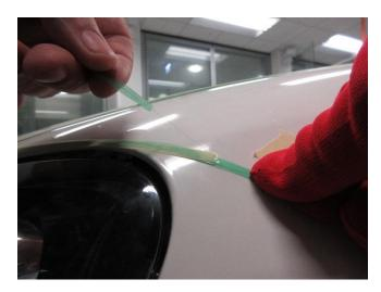
Fold the filament over the Cover Tape and press your thumb on it.
