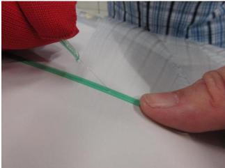
Tack end of filament to vehicle until ready to cut film.
