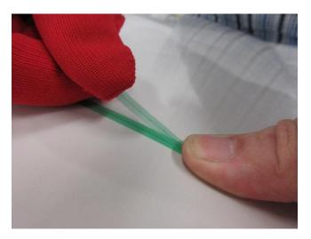
Firmly grasp the end of the tape with your thumb and index finger positioning your two thumbs close together to start the filament. Gently pull the line to tear the carrier tape and expose the filament.
