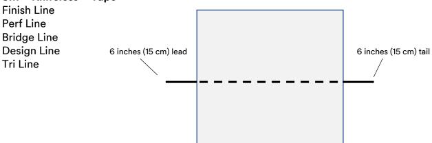
Begin with 6 inches (15 cm) of tape (before and after) where the graphic will be cut and lay down 3M<sup>™</sup> Knifeless<sup>™</sup> Tape. Apply the film with pressure over the 3M<sup>™</sup> Knifeless<sup>™</sup> Tape, leaving the lead and tail tape visible.
