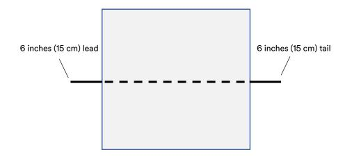
Begin with 6 inches (15 cm) of tape (before and after) where the graphic will be cut and lay down 3M™ Knifeless™ Tape. Apply tape everywhere film will be cut.
