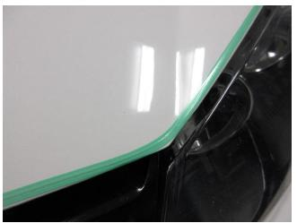
Start all lines (both lead and tail) by folding the start of the tape back over itself approximately 3 inches (8 cm) and press thumb firmly on folded edge, covering at least 0.4 inches (1 cm) tape.
