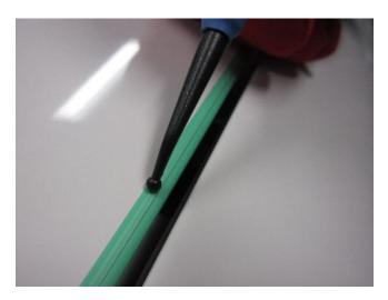
Apply the paint protection film with firm pressure over the tape, leaving the lead and tail tape visible, according to wet application instructions. The use of installation gel is recommended.
