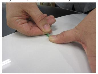
Pull the line back and not upward, stopping before the edge of the graphic.
