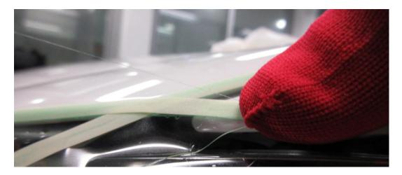
Tug the filament to start cutting, continuing to pull the line back and not upward in direction of the cut line.
