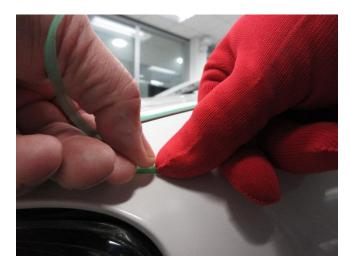
Gently pull the line to tear the carrier tape and expose the filament. Tack end of filament to vehicle until ready to cut film.
