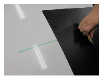
To remove air bubbles, press the film onto the 3M™ Knifeless™ Tape again with your finger.
