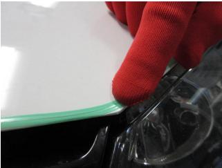
The use of special application tools helps to remove air underneath the tape.
