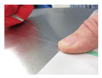
Gently tug the filament to start cutting into the graphic, continuing to pull the line back and not upward in direction of the cut line.
