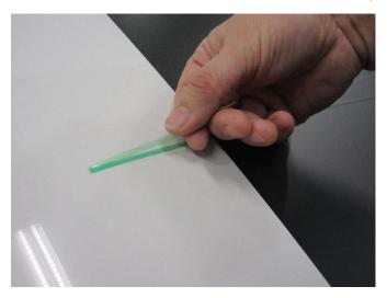
Press thumb firmly on folded edge, covering at least 0.4 inches (1 cm) tape. Firmly grasp the end of the tape with your thumb and index finger. Start with your two thumbs 0.4 inches (1 cm) apart. Bring thumbs together and give the tape a quick snap, breaking the carrier tape and exposing the filament (line).
